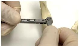
Fig. 3: Loosening the socket screw by turning it to the left
